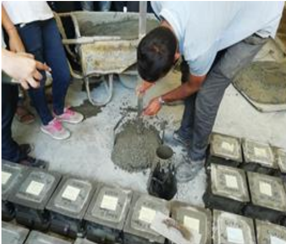
Slump cone test for fresh concrete
